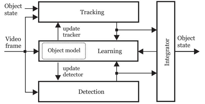
Fig. 8. Detailed block diagram of the TLD framework.
