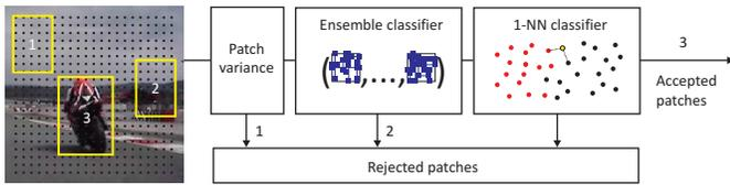
Fig. 9. Block diagram of the object detector.
