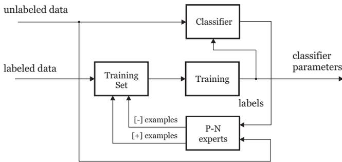
Fig. 3. The block diagram of the P-N learning.
