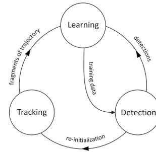
Fig. 2. The block diagram of the TLD framework.
