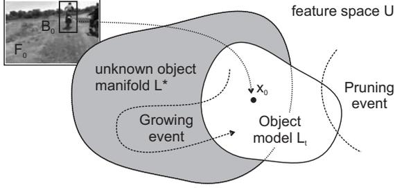
Figure 1. The online model is initialized in the first frame by the selected sample  $x_0$ . It is expanding by “growing events”, refined by “pruning events” and slowly converges toward the unknown object manifold.
